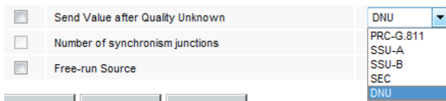
Figure 5-27: Synchronism Status Message Combo Box
