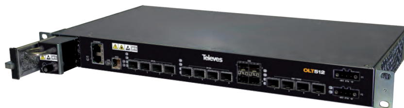
Figure 4-5: OLT cooling module with redundant FANS
